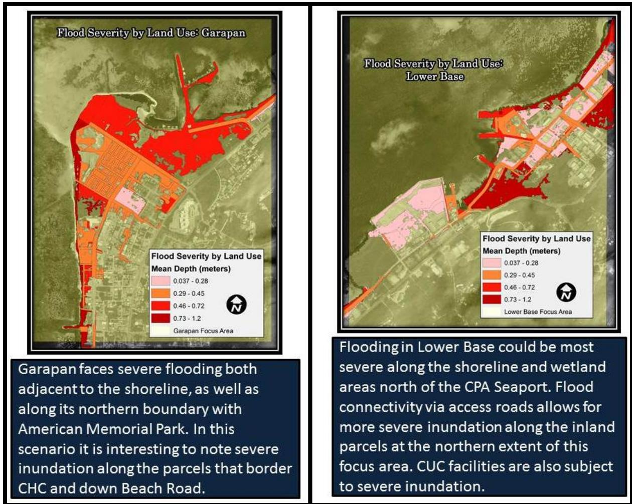
**Figure 5-14 Flood Severity in Garapan and Lower Base, Saipan**
